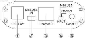
① USB Port: These ports are the converter's USB Hub provision that allows user to connect a USB Hard Drive, USB web camera, Keyboard or Mouse.
